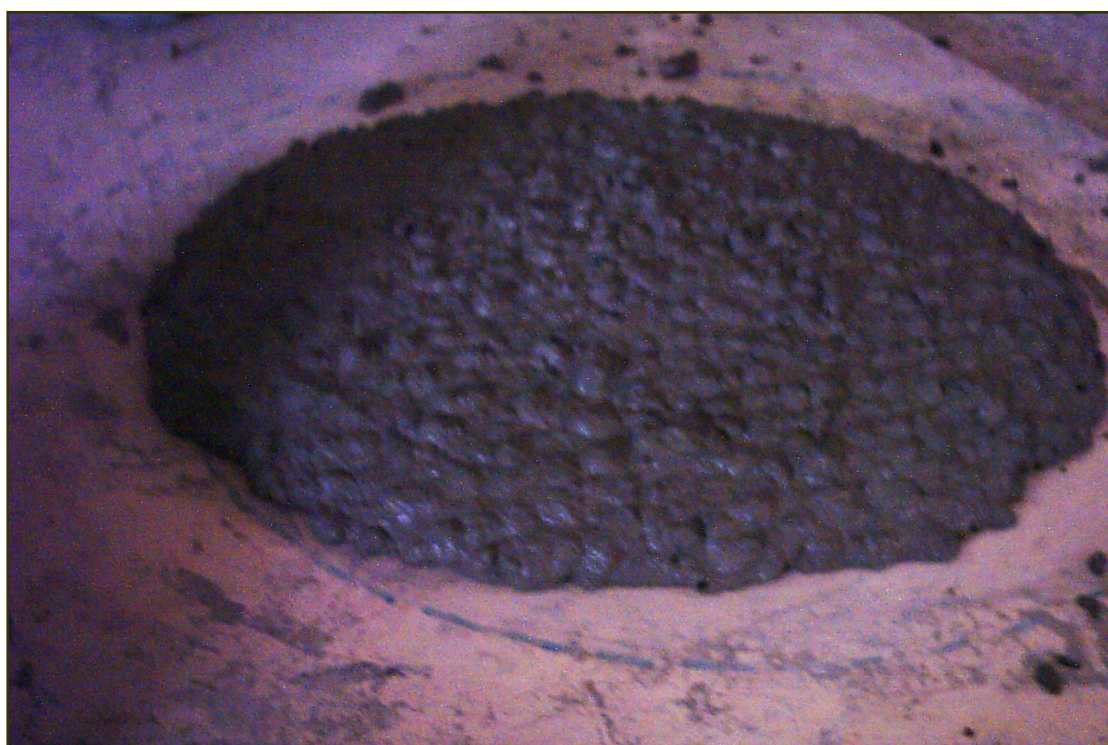
Fig. (1) Flow Test of SCC concrete.
